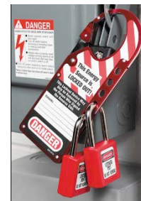
Panel and breaker locks
